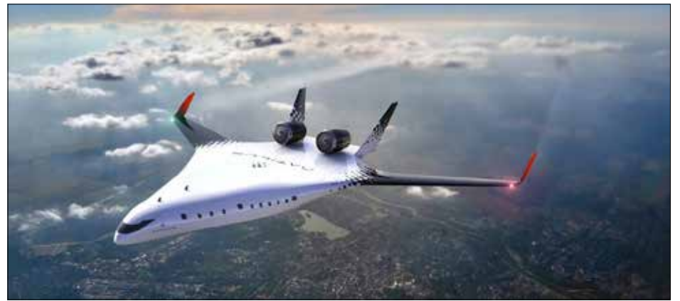
The 200-passenger Horizon is the latest addition to Natilus's family of blended wing body aircraft, which delivers exceptional fuel efficiency and higher payloads. Rendering courtesy Natilus Inc.
